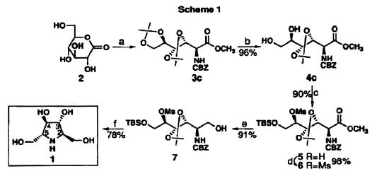
Reagents: (a) ref. 8 (b) Dowex 50W-X8 (H+), 90% methanol, rt (c) TBDMSCl, imidazol, DMF, 0°C (d) MsCl, THF, rt (e) LiAlH<sub>4</sub>, THF, 0°C (f) i) Dowex 50W-X8, 95% methanol, reflux ii) sodium acetate, Pd/C, methanol.
